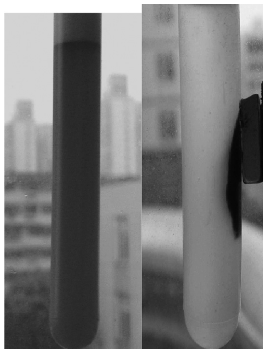
Fig. 7. Shows the attraction of the nanospheres to a 0.5 T magnet.
